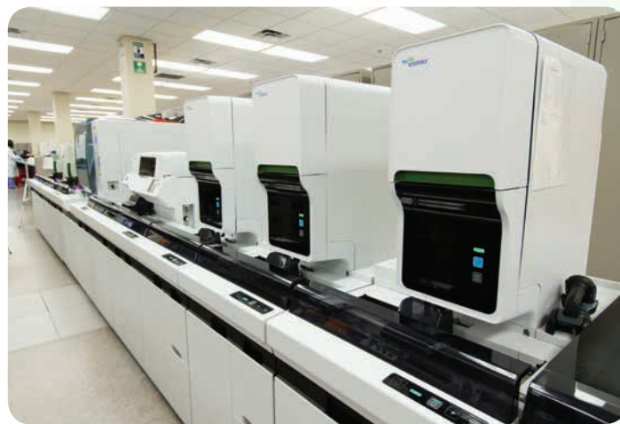
The Sysmex XN-9000 Lavender Top Management System equipped with Bio-Rad VARIANT™ II TURBO Link analyzer provide RML with fully automated CBC and A1c testing powered by Sysmex WAM.
